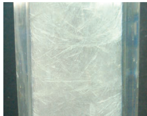
Figure 6. EGPA coarse crystal (mixture of \text{H}_3\text{PO}_4 \cdot 0.5\text{H}_2\text{O} crystal and phosphoric acid aqueous solution).
